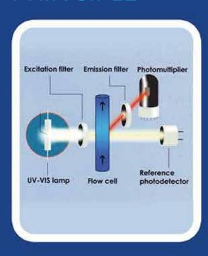
The measuring principle is based on fluorescence: when light at a specific wavelength (excitation), some chemicals re-emit (emission) at a longer wavelength.
