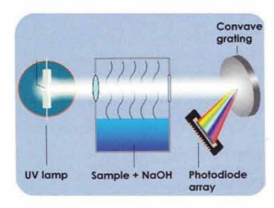
The measuring principle is based on UV light absorption spectrum of ammonia gas NH3 in equilibrium with dissolved ammoniac gas in the water sample.
